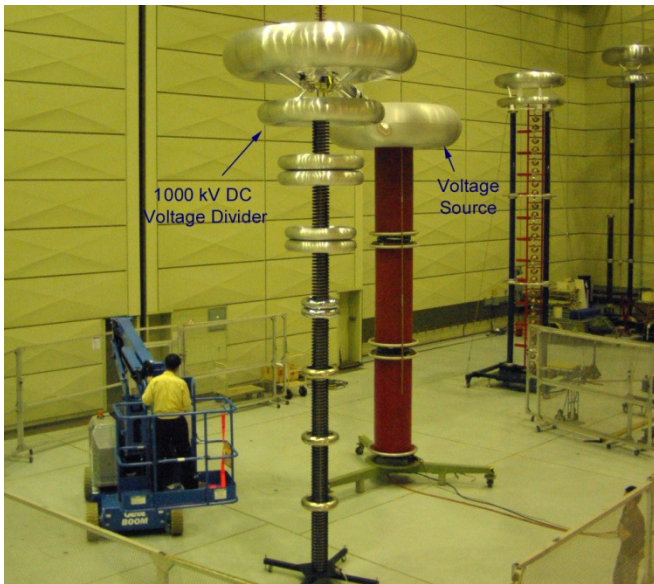
1000 kV DC divider with measurement uncertainty of 100 \mu\text{V/V}
