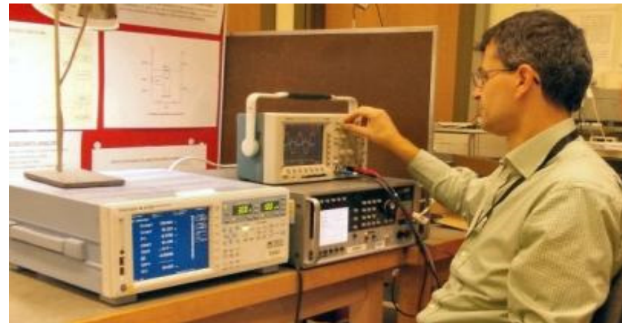
Calibration of a wideband wattmeter for use in LED power measurements with distorted current waveforms.
