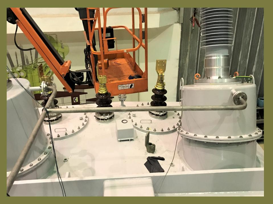
Stainless Steel Pipework, Sloping Lid, Zinc Spray Main Tank
