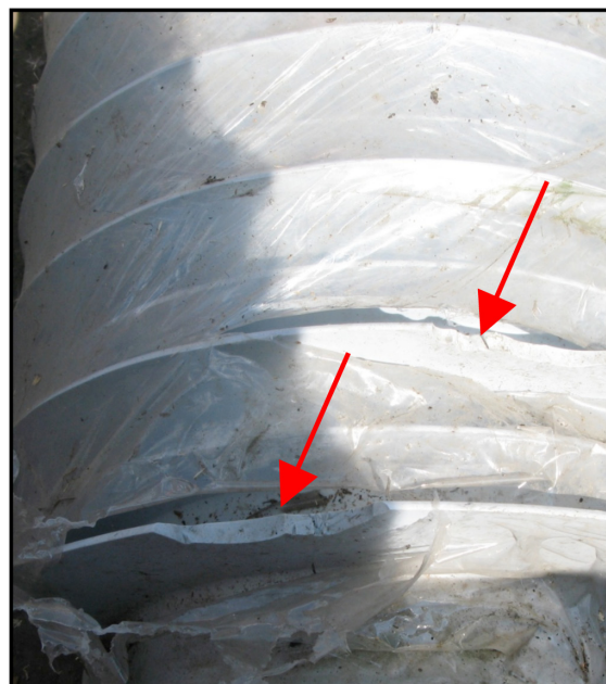
Figure 6.5: Example of rodent attack on the silicone sheds after 10 years storage in the original package (marked with red arrows)
