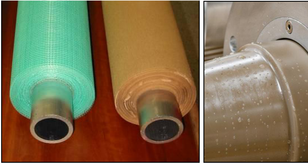
Figure 2.2.1: RIS and OIP bushing unimpregnated condenser body (left), RIS high hydrophobicity (right)
