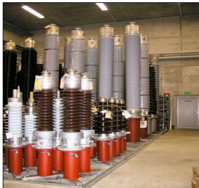
Figure 6.3: Example of long-term storage of various bushing types, [3.2.8]
