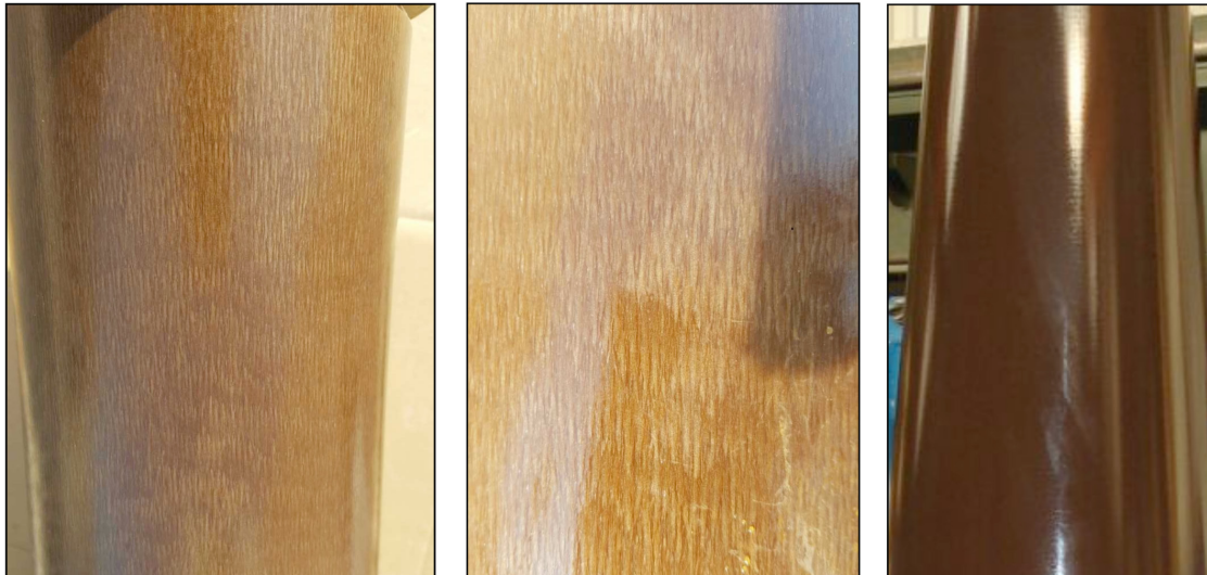
Figure 6.1: RIP bushing's oil part visual appearance; left: humidified body, centre: humidified body – enlarged, right: dry
