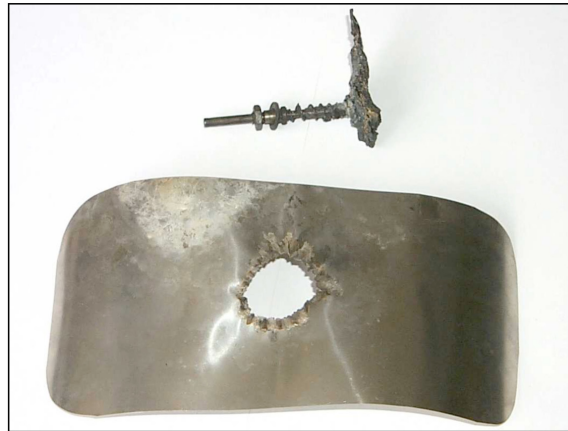
Figure 4.1.1.2: Arcing traces on last electrode and tap elements
