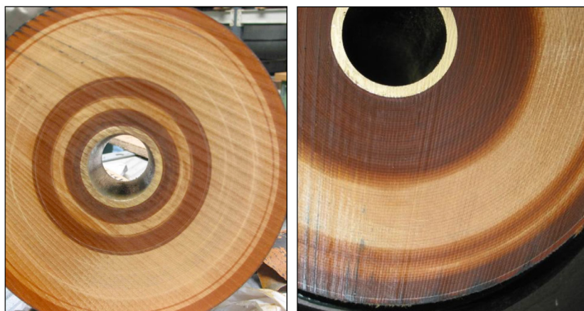
Figure 4.1.3.2: Two examples of oil penetration into RBP bushing condenser body (darker area)
