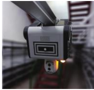
(a) rail-based robot (Source: courtesy of State Grid Corporation of China)
